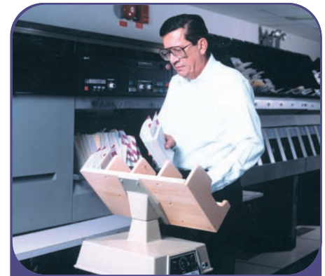
Syntron® J-50 4-pocket, shown here, aligning checks prior to insertion into the Lundy Machine.
