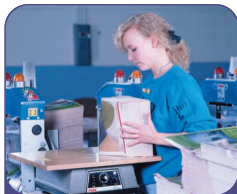
The Model J-50 flat deck enables this worker at a major daily newspaper to quickly aerate and align magazine inserts prior to loading into the inserting machines.
